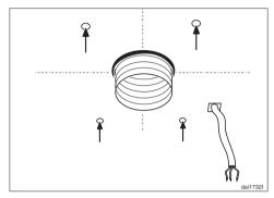
Drill four <sup>3</sup>/<sub>16</sub>" (5 mm) holes in the ceiling.
